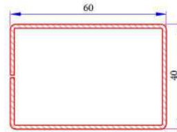
Super Mullion Reinforcement Code: 34022-12110
