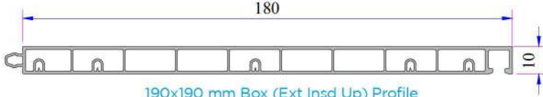
190x190 mm Box (Ext Insd Up) Profile Code: P.A.097.5601.600.0.00.19
